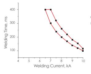
Weld lobe of Galvano<sup>™</sup> (0.8 mm). Coating weight: 120gsm
